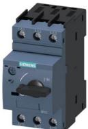
Circuit breaker size S0 for motor protection, CLASS 10 A-release 9...12.5 A N-release 163 A screw terminal Standard switching capacity
